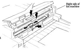
**6** Gently close the scanner cover, making sure both sides are snapped down securely.
